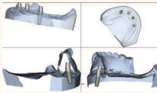
Figure 7. Design images showing the contour and tooth position of the duplicate denture and proposed design of the ATLANTIS Conus Abutments
