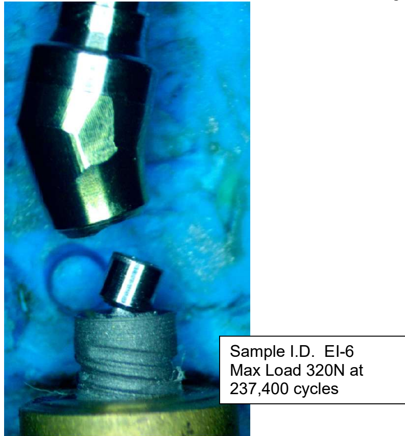
Figure 7 - Fatigue Test Failure Mode – Abutment crack at top of hex & abutment screw yielding.
