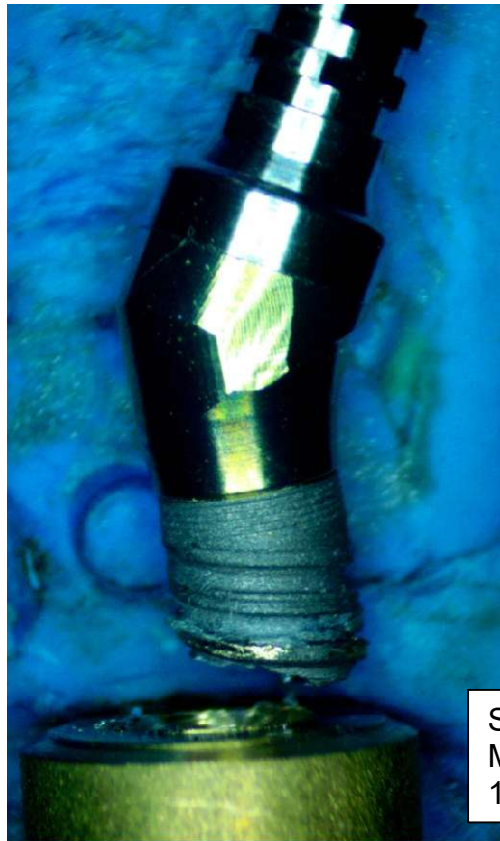
Figure 5 - Fatigue Test Failure Mode – Implant crack below pot line and abutment screw failure
