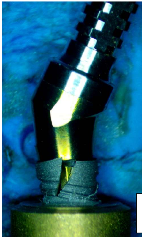
Figure 6 - Fatigue Test Failure Mode – Vertical crack in implant collar.
