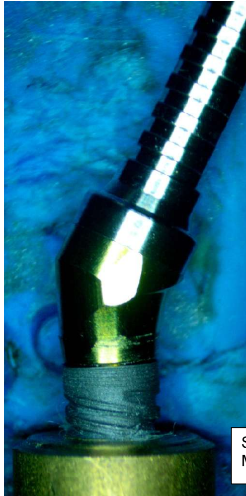
Figure 3 - Static Compression Test Failure Mode – Bellmouth yielding of implant collar
